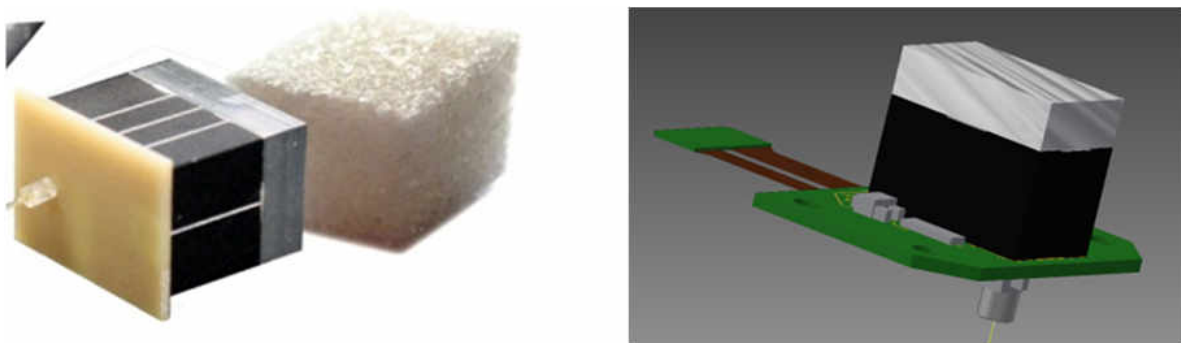
Figure 5-Left: the sugar-cube sized NIR spectrometer. Right: Design drawing of the spectrometer on its read-out board.
